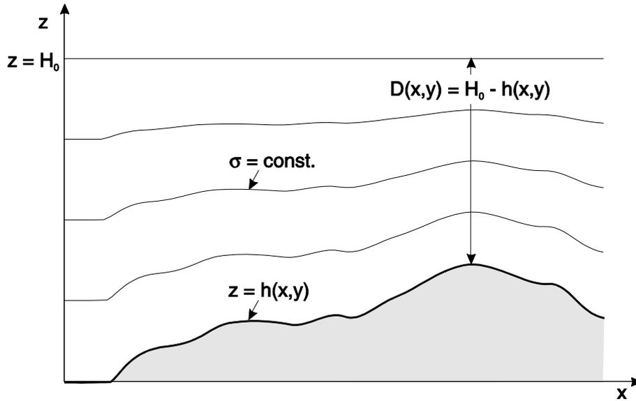
Figure 4: A schematic representation of the vertical extent of the model domain and the position of the model layers, when the terrain following coordinate transform is applied.
